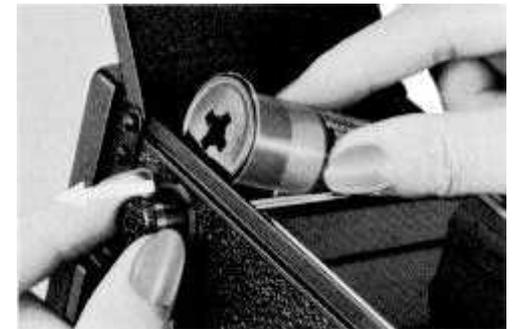
\* - To minimize the trouble in loading your next film, it is advisable to take out the empty spool from the lower film chamber and to set it in the upper chamber immediately after unloading the exposed film.
