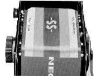
6 - After ascertaining that the trimmed edge of the film leader rests flush against the edge of the slot, turn the Film Wind Crank-handle gently in the direction of the arrow and check whether the film is advancing properly.
