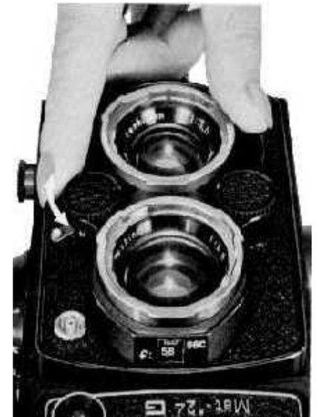
\* When the yellow follower needle (Y) perfectly coincides with the meter pointer (I), it signifies that THE CAMERA is set for correct exposure. The proper combination of the shutter speed and aperture is shown in the Shutter Speed and Aperture Indicator Windows.
