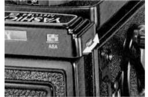
2 - Center the desired shutter speed in the Shutter Speed Indicator Window by turning the Shutter Speed Control Dial. The exposure meter pointer in the Exposure Indicator Window is coupled to the shutter mechanism and will shift in either direction when the shutter speed is adjusted.
