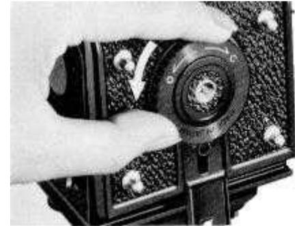
3 - Pull out the Upper Spool Holder Knob and take out the exposed film from the film chamber. Paste the seal to prevent recoiling and wrap the film in light-proof paper.
