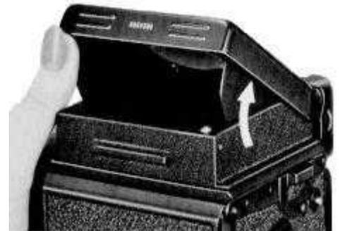
\* When the camera is to be left unused, fold the focusing hood. This will switch off the meter and prevent draining of battery power.
