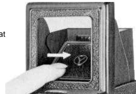
To close the Cover, push the Release Button on the back of the Focusing Hood.
