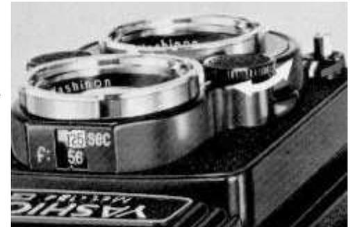
3 - The exposure meter begins to function when the focusing hood is set upright by lifting it up gently with your fingertip.
