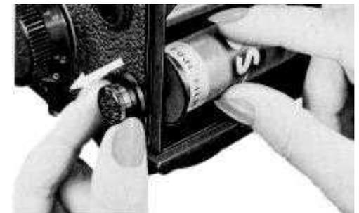
5 - Draw out the film leader gently and introduce its tip straight and amply into the slot on the spindle of the Take-up Spool. The film may fail to advance if the film leader is not inserted properly into the slot.
